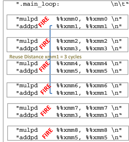
Figure 2. Microbenchmark for testing instruction latencies.
