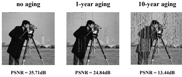
Fig. 1. Impact of the aging-induced delay in an image processing application.
